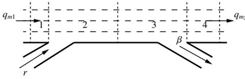
Fig. 1. A schematic plot of a 4-cell freeway section with one on-ramp and one off-ramp.
