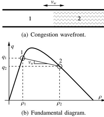
Fig. 4. The fundamental diagram and congestion wavefront propagation.
